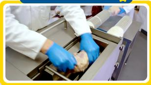
Reduce downtime and achieve a consistent output of 1200 units per hour – one operator cuts the netted joint while the loader simultaneously refills the chamber to ensure efficient workflow.
